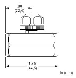
SUN adjustable gage snubbers are throttling and shut-off devices used to isolate and protect hydraulic gages from line pressure transients and the resulting gage pointer pulsations.
