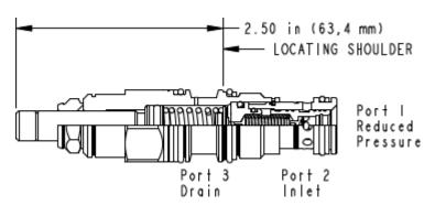
Pilot-operated, pressure reducing valves reduce a high primary pressure at the inlet (port 2) to a constant reduced pressure at port 1, allowing circuits with multiple pressure requirements to be operated using a single pump.
