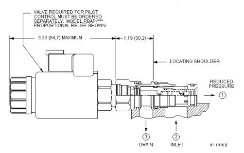
This valve is a normally open modulating element that incorporates an integral pilot control cavity. The pilot control cavity will accept any T-8A pressure control cartridge. The valve reduces a high primary pressure at the inlet (port 2) to a constant reduced pressure at port 1. The pilot cartridge's setting determines the difference in pressure between reduced pressure (port 1) and the drain (port 3).
