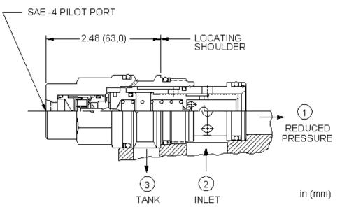
Air-controlled, pilot-operated pressure reducing cartridges use compressed air over a diaphragm instead of an adjustable spring as the setting to reduce a high primary pressure at the inlet (port 2) to a constant reduced pressure at port 1. The air signal is supplied through a port in the hex-end of the cartridge and the hydraulic setting is directly proportional to the air setting at a ratio of 20:1 (hydraulic:air).
