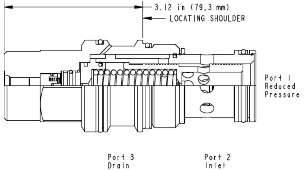
Air-controlled, pilot-operated pressure reducing cartridges use compressed air over a diaphragm instead of an adjustable spring as the setting to reduce a high primary pressure at the inlet (port 2) to a constant reduced pressure at port 1. The air signal is supplied through a port in the hex-end of the cartridge and the hydraulic setting is directly proportional to the air setting at a ratio of 20:1 (hydraulic:air).
