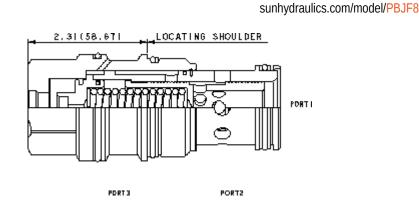
This valve is a normally open modulating element that incorporates an integral pilot control cavity. The pilot control cavity will accept any T-8A pressure control cartridge. The valve reduces a high primary pressure at the inlet (port 2) to a constant reduced pressure at port 1. The pilot cartridge's setting determines the difference in pressure between reduced pressure (port 1) and the drain (port 3).
