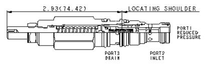
Pilot-operated, pressure reducing/relieving valves reduce a high primary pressure at the inlet (port 2) to a constant reduced pressure at port 1, with a full-flow relief function from port 1 to tank (port 3).
