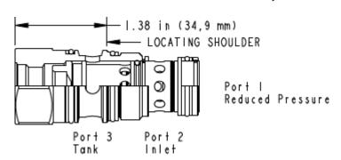
This valve is a 3-way, normally open modulating element that incorporates an integral pilot control cavity. The pilot control cavity will accept any T-8A pressure control cartridge. The valve reduces a high primary pressure at the inlet (port 2) to a constant reduced pressure at port 1, with a full flow relief function from port 1 to tank (port 3). The pilot cartridge's setting determines the difference in pressure between reduced pressure (port 1) and the tank (port 3).
