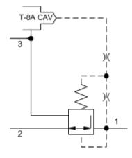
VALVE REQUIRED FOR PILOT CONTROL MUST BE ORDERED SEPARATELY. MODEL RBAP-\*\*\* PROPORTIONAL RELIEF SHOWN. 3.33 (84,7) MAXIMUM - 1.81 (46,0) LOCATING SHOULDER REDUCED Ħ PRESSURE II IL™ (1)⊕ EC 2 3 2 TANK INLET in. (mm)
