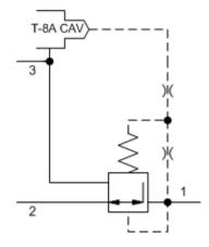
VALVE REQUIRED FOR PILOT CONTROL MUST BE ORDERED SEPARATELY. MODEL RBAP-\*\*\* PROPORTIONAL RELIEF SHOWN. 3.33 (84,7) MAXIMUM – 2.31 (58,7) – – – LOCATING SHOULDER REDUCED PRESSURE  $\sim$  $\overline{\mathbf{n}}$  $\overline{O}$  $\overline{\Omega}$ -Đ l d h (1)⊕ 3 (2)TANK INLET in. (mm)
