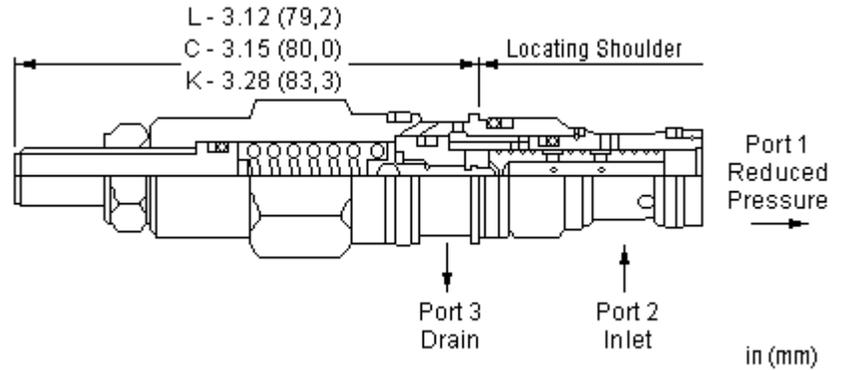
Direct-acting, pressure reducing valves reduce a high primary pressure at the inlet (port 2) to a constant reduced pressure at port 1. These valves incorporate a damped construction for stable operation allowing the use of high reduced pressure. This valve is open in the transition from reducing to relieving. It provides good pressure control and dynamic response.
