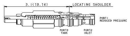
Direct-acting, pressure reducing valves reduce a high primary pressure at the inlet (port 2) to a constant reduced pressure at port 1. These valves incorporate a damped construction for stable operation allowing the use of high reduced pressure.
