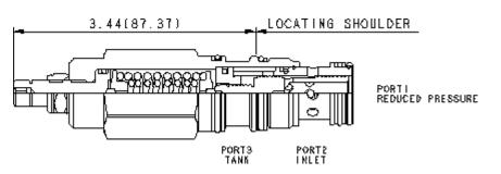
Direct-acting, pressure reducing valves reduce a high primary pressure at the inlet (port 2) to a constant reduced pressure at port 1. These valves incorporate a damped construction for stable operation allowing the use of high reduced pressure.
