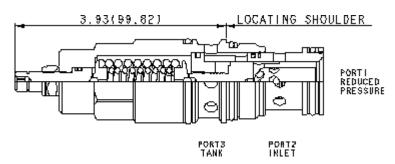
Direct-acting, pressure reducing/relieving valves reduce a high primary pressure at the inlet (port 2) to a constant reduced pressure at port 1, with a full-flow relief function from port 1 to tank (port 3). These valves incorporate a damped construction for stable operation allowing the use of high reduced pressure.
