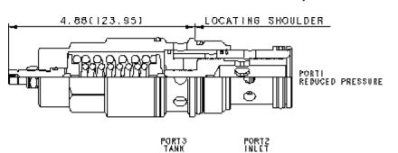
Direct-acting, pressure reducing/relieving valves reduce a high primary pressure at the inlet (port 2) to a constant reduced pressure at port 1, with a full-flow relief function from port 1 to tank (port 3). These valves incorporate a damped construction for stable operation allowing the use of high reduced pressure.
