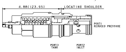
Direct-acting, pressure reducing valves reduce a high primary pressure at the inlet (port 2) to a constant reduced pressure at port 1. These valves incorporate a damped construction for stable operation allowing the use of high reduced pressure.
