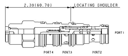
The direct-acting reducer/reliever main section is meant to act as an interface between a low flow pressure source at port 4 and a circuit with higher flow requirements. The valve will reduce a high primary pressure at the inlet (port 2) to a reduced pressure at port 1, with a full-flow relief function from port 1 to tank (port 3). The valve incorporates a damped construction for stable operation allowing the use of high reduced pressure.
