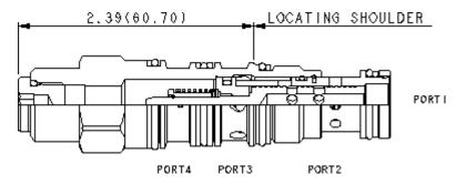
The direct-acting reducer/reliever main section is meant to act as an interface between a low flow pressure source at port 4 and a circuit with higher flow requirements. The valve will reduce a high primary pressure at the inlet (port 2) to a reduced pressure at port 1, with a full-flow relief function from port 1 to tank (port 3). The valve incorporates a damped construction for stable operation allowing the use of high reduced pressure.
