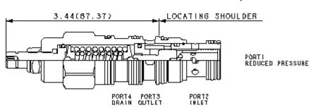
Direct-acting, pressure reducing/relieving valves reduce a high primary pressure at the inlet (port 2) to a constant reduced pressure at port 1, with a full-flow relief function from port 1 to tank (port 3). Draining port 4 makes the valve insensitive to pressure at port 3. These valves incorporate a damped construction for stable operation allowing the use of high reduced pressure.
