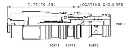
The direct-acting reducer/reliever main section is meant to act as an interface between a low flow pressure source at port 4 and a circuit with higher flow requirements. The valve will reduce a high primary pressure at the inlet (port 2) to a reduced pressure at port 1, with a full-flow relief function from port 1 to tank (port 3). The valve incorporates a damped construction for stable operation allowing the use of high reduced pressure.
