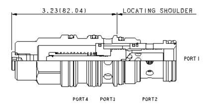
The direct-acting reducer/reliever main section is meant to act as an interface between a low flow pressure source at port 4 and a circuit with higher flow requirements. The valve will reduce a high primary pressure at the inlet (port 2) to a reduced pressure at port 1, with a full-flow relief function from port 1 to tank (port 3). The valve incorporates a damped construction for stable operation allowing the use of high reduced pressure.
