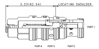
The direct-acting reducer/reliever main section is meant to act as an interface between a low flow pressure source at port 4 and a circuit with higher flow requirements. The valve will reduce a high primary pressure at the inlet (port 2) to a reduced pressure at port 1, with a full-flow relief function from port 1 to tank (port 3). The valve incorporates a damped construction for stable operation allowing the use of high reduced pressure.
