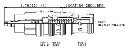
Externally drained, pilot-operated pressure reducing/relieving valves reduce a high primary pressure at the inlet (port 2) to a constant reduced pressure at port 1, with a full-flow relief function from port 1 to tank (port 3). Draining the pilot section at port 4 makes these valves insensitive to pressure at tank (port 3) and provides a means for remote control by pilot or 2-way valves.
