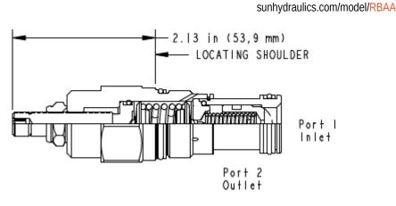
Direct-acting, pilot relief cartridges are used to remotely control the pressure setting of other pilot-operated valves. Because capacity is limited to pilot flow, these valves should be used with other higher flow valves.
