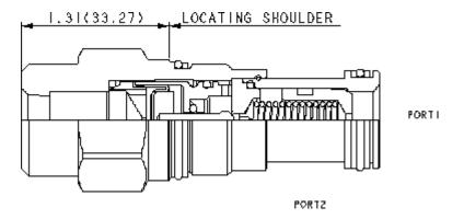
Air-controlled, pilot relief cartridges are used to remotely control the pressure setting of other pilot operated valves. Because capacity is limited to pilot flow, these valves should be used with valves with compatable pilot flows. They use compressed air over a diaphragm instead of an adjustable spring to control pressure setting, the air signal is supplied through a port in the hex-end of the cartridge.
