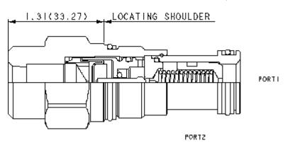
Air-controlled, pilot relief cartridges are used to remotely control the pressure setting of other pilot operated valves. Because capacity is limited to pilot flow, these valves should be used with valves with compatable pilot flows. They use compressed air over a diaphragm instead of an adjustable spring to control pressure setting, the air signal is supplied through a port in the hex-end of the cartridge.
