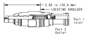
Direct-acting, pilot relief cartridges are used to remotely control the pressure setting of other pilot-operated valves. Because capacity is limited to pilot flow, these valves should be used with other higher flow valves.
