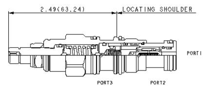
This direct-acting, pilot relief cartridge incorporates back-to-back check valves. This allows it to remotely control 2 other pilot-operated valves or act as a thermal relief for both ends of an actuator. Because capacity is limited to pilot flow, this valve should be used with other valves with comparable pilot flows.
