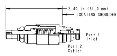
Two-port, pilot-stage, direct-acting relief cartridges are fully adjustable, normally closed pressure regulating valves. When the pressure at port 1 (inlet) is sufficient to overcome the spring force (valve setting), a flow path is opened from port 1 to port 2 (tank).
