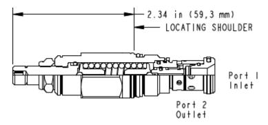
The bi-directional, direct-acting relief cartridge is a normally closed, pressure-limiting valve used to protect hydraulic components from pressure transients. When the pressure differential between ports 1 and 2 exceeds the valve setting, the valve starts to open, throttling flow to limit the pressure rise, regardless of the direction.
