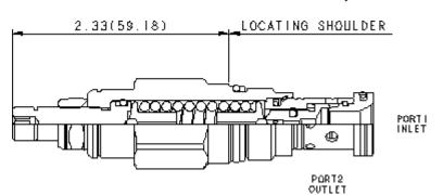
Direct-acting relief cartridges are normally closed, pressurelimiting valves used to protect hydraulic components from pressure transients. When the pressure at the inlet (port 1)
