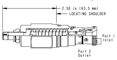
Direct-acting relief cartridges are normally closed, pressurelimiting valves used to protect hydraulic components from
