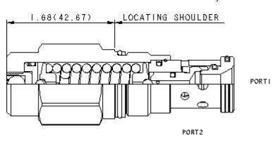
Non-adjustable direct-acting relief cartridges are normally closed, pressure-limiting valves used to protect hydraulic components from pressure transients. When the pressure at the inlet (port 1) reaches the valve setting, the valve starts to open to tank (port 2), throttling flow to limit the pressure rise. These valves are smooth and quiet, essentially zero leak, dirt tolerant, immune to silting and are very fast.
