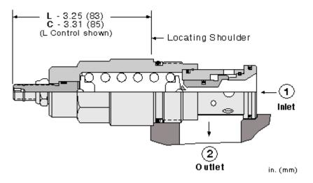
Direct-acting relief cartridges are normally closed, pressure-limiting valves used to protect hydraulic components from pressure transients. When the pressure at the inlet (port 1) reaches the valve setting, the valve starts to open to tank (port 2), throttling flow to limit the pressure rise. These valves are smooth and quiet, essentially zero leak, dirt tolerant, immune to silting and are very fast.
