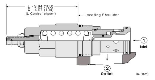
Direct-acting relief cartridges are normally closed, pressure-limiting valves used to protect hydraulic components from pressure transients. When the pressure at the inlet (port 1) reaches the valve setting, the valve starts to open to tank (port 2), throttling flow to limit the pressure rise. These valves are smooth and guiet, essentially zero leak, dirt tolerant, immune to silting and are very fast.
