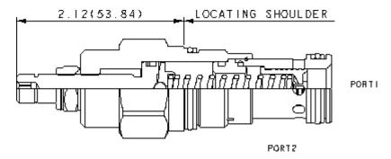
Direct-acting relief cartridges are normally closed, pressure-limiting valves used to protect hydraulic components from pressure transients. When the pressure at the inlet (port 1) reaches the valve setting, the valve starts to open to tank (port 2), throttling flow to limit the pressure rise.
