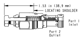
Pilot-operated, balanced-piston relief cartridges are normally closed pressure regulating valves. When the pressure at the inlet (port 1) reaches the valve setting, the valve starts to open to tank (port 2), throttling flow to regulate the pressure. These valves are accurate, have low pressure rise vs. flow, they are smooth and quiet, and are moderately fast.
