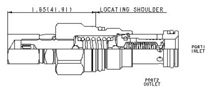
Pilot-operated, balanced-piston relief cartridges are normally closed pressure regulating valves. When the pressure at the inlet (port 1) reaches the valve setting, the valve starts to open to tank (port 2), throttling flow to regulate the pressure. These valves are accurate, have low pressure rise vs. flow,
