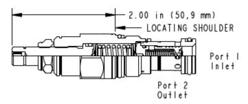
Pilot-operated, balanced-piston relief cartridges are normally closed pressure regulating valves. When the pressure at the inlet (port 1) reaches the valve setting, the valve starts to open to tank (port 2), throttling flow to regulate the pressure. These valves are accurate, have low pressure rise vs. flow, they are smooth and quiet, and are moderately fast.
