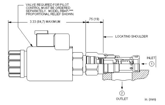
This valve is a normally closed modulating element that incorporates an integral pilot control cavity. It is a balanced piston design. The pilot control cavity will accept any T-8A pressure control cartridge. When the pressure at the inlet (port 1) reaches the pilot control cartridge's setting, the modulating element starts to open to tank (port 2), throttling flow to regulate the pressure. The pilot cartridge's setting determines the difference in pressure between port 1 and port 2.
