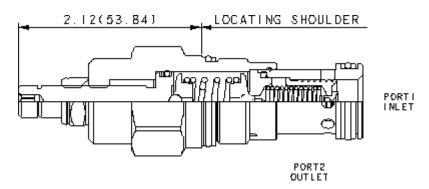
Pilot-operated, balanced-piston relief cartridges are normally closed pressure regulating valves. When the pressure at the inlet (port 1) reaches the valve setting, the valve starts to open to tank (port 2), throttling flow to regulate the pressure. These valves are accurate, have low pressure rise vs. flow,
