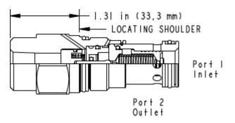
Air-controlled, pilot-operated, balanced piston relief cartridges use compressed air over a diaphragm instead of an adjustable spring to control pressure setting. The air signal is supplied through a port in the hex-end of the cartridge. They are normally closed pressure regulating valves. When the pressure at the inlet (port 1) reaches the valve setting, the valve starts to open to tank (port 2), throttling flow to regulate the pressure. These valves are
