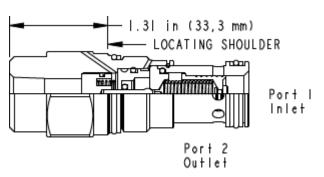
Air-controlled, pilot-operated, balanced piston relief cartridges use compressed air over a diaphragm instead of an adjustable spring to control pressure setting. The air signal is supplied through a port in the hex-end of the cartridge. They are normally closed pressure regulating valves. When the pressure at the inlet (port 1) reaches the valve setting, the valve starts to open to tank (port 2), throttling flow to regulate the pressure. These valves are
