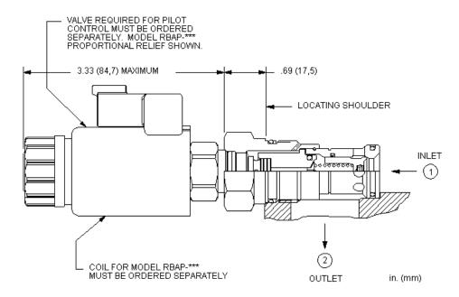
This valve is a normally closed modulating element that incorporates an integral pilot control cavity. It is a balanced poppet design. The pilot control cavity will accept any T-8A pressure control cartridge. When the pressure at the inlet (port 1) reaches the pilot control cartridge's setting, the poppet element starts to open to tank (port 2), throttling flow to regulate the pressure. The pilot cartridge's setting determines the difference in pressure between port 1 and port 2.
