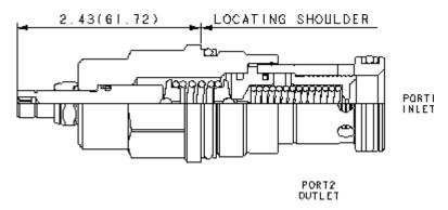
Pilot-operated, balanced-piston relief cartridges are normally closed pressure regulating valves. When the pressure at the inlet (port 1) reaches the valve setting, the valve starts to open to tank (port 2), throttling flow to regulate the pressure. These valves are accurate, have low pressure rise vs. flow,
