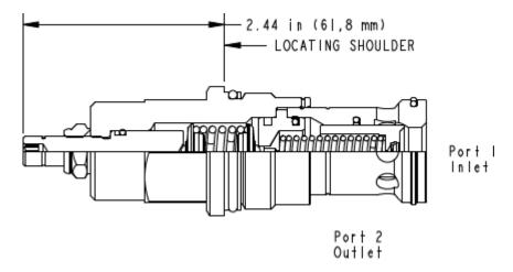
Pilot-operated, balanced-poppet relief cartridges are normally closed pressure regulating valves. When the pressure at the inlet (port 1) reaches the valve setting, the valve starts to open to tank (port 2), throttling flow to regulate the pressure. These valves are accurate, smooth, quiet, fast, and have low pressure rise vs. flow.
