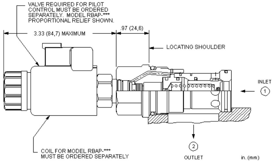
This valve is a normally closed modulating element that incorporates an integral pilot control cavity. It is a balanced poppet design. The pilot control cavity will accept any T-8A pressure control cartridge. When the pressure at the inlet (port 1) reaches the pilot control cartridge's setting, the poppet element starts to open to tank (port 2), throttling flow to regulate the pressure. The pilot cartridge's setting determines the difference in pressure between port 1 and port 2.
