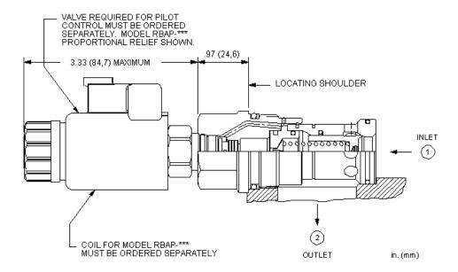
This valve is a normally closed modulating element that incorporates an integral pilot control cavity. It is a balanced poppet design. The pilot control cavity will accept any T-8A pressure control cartridge. When the pressure at the inlet (port 1) reaches the pilot control cartridge's setting, the poppet element starts to open to tank (port 2), throttling flow to regulate the pressure. The pilot cartridge's setting determines the difference in pressure between port 1 and port 2.
