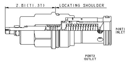
Fast-acting, pilot-operated, balanced piston relief cartridges are normally closed, pressure-limiting valves used to protect hydraulics components from pressure transients. Fast opening and closing is gained at the expense of smoothness. When the pressure at the inlet (port 1) reaches the valve setting, the valve starts to open to tank (port 2), throttling flow to limit the pressure rise. These valves have low pressure rise vs. flow and are very fast.
