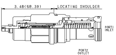
Pilot-operated, anti shock relief cartridges limit maximum system pressure and also limit the rate of pressure rise. The valve opens and then ramps closed at a constant speed, independent of settings and flows. The adjust screw determines the maximum (relief) setting and the minimum (threshold) setting.
